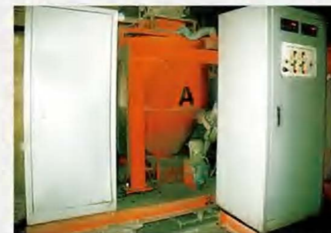
Burnt Brick Batching System
