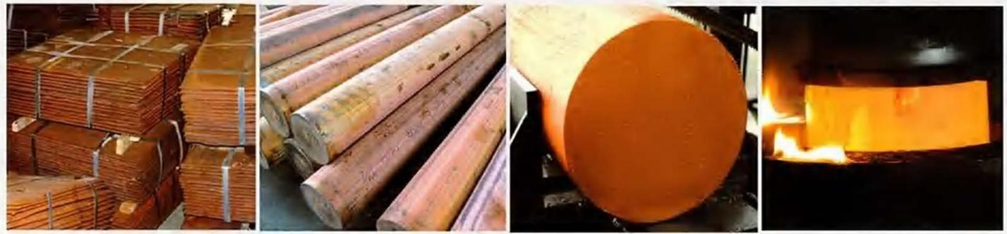
TP2 is a kind of material is selected by most of the steel plants. It shows excellent heat-proof and anti-fatigue property under high temperature and it has good processing property.
